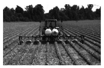
Figure 7. Shielded sprayer in soybeans
