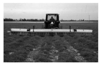
Figure 6. Broadcast shielded sprayer operating in "burn-down"
